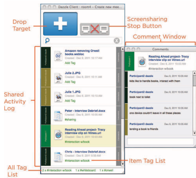
Figure 4: The Dazzle interface shows a drop target, a shared activity log, and a comment window.
