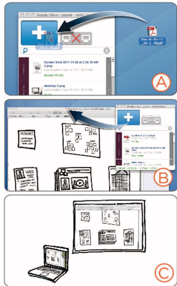
Figure 3: To bring a file to others' attention, the participant drags that file on to the drop target (A). This opens the file locally on that person's computer (B), as well as initiates screensharing with a public display (C).
