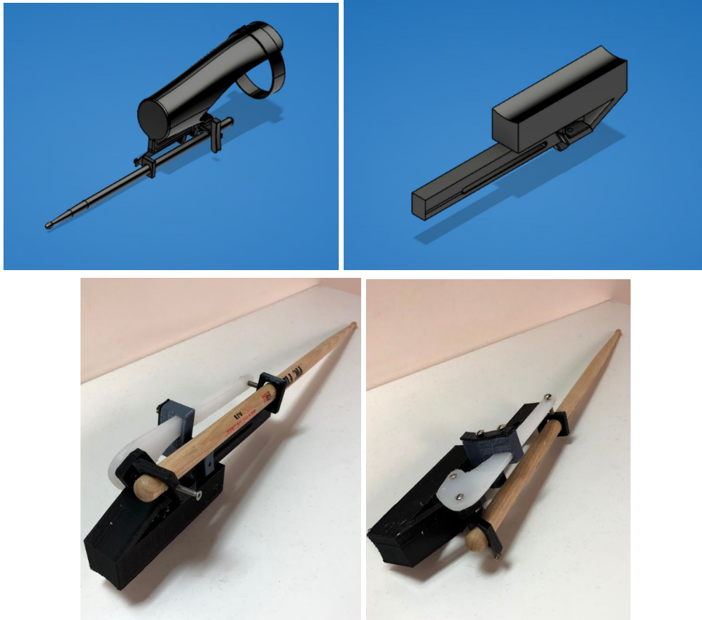
Figures 14-17: Original Paradiddle design (Upper Left), modified Paradiddle design without the built-in socket (Upper Right), Paradiddle Prototype Top View (Lower Left), Paradiddle Prototype Side View (Lower Right)
