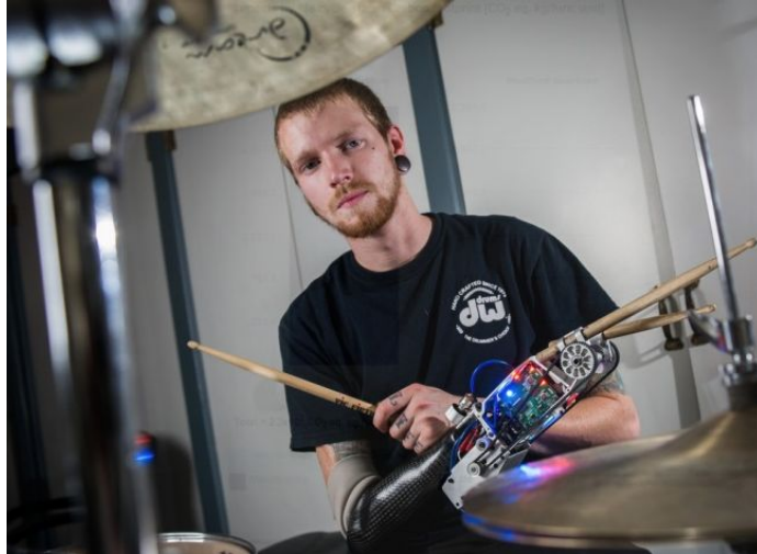
Figure 1: Georgia Tech Myoelectric Drumming Prosthesis (Bretan, M., Gopinath, D., Mullins, P. & Weinberg, G. A Robotic Prosthesis for an Amputee Drummer. arXiv:1612.04391 [cs] (2016)).
