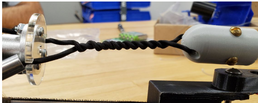
Figure 24: Stiff conformation for the Twisted String Actuated Prototype
