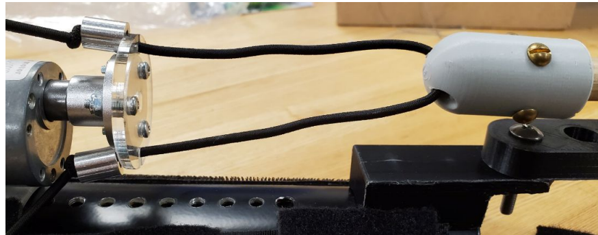
Figure 23: Nonstiff conformation for the Twisted String Actuated Prototype
