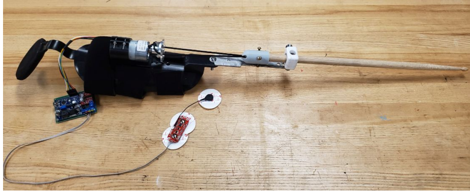
Figure 22: Twisted String Prototype with electronics
