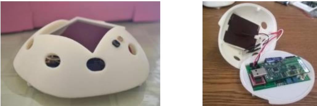
*Figure 8: Abalone wireless sensor fully assembled (left) and showing internal circuitry (right)*
