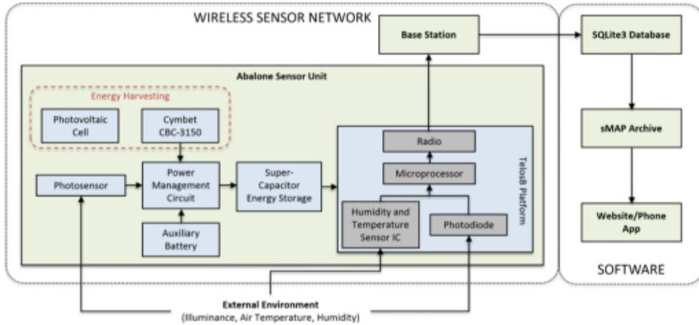
Figure 9: System diagram of wireless sensor network and communication protocol
