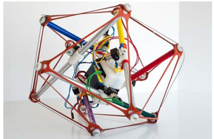
**FIGURE 1:** The TT-4<sub>mini</sub> prototype, the first tensegrity robot that uses the elastic lattice platform. This robot moves by adjusting the lengths of its cables with respect to its elastic lattice.
