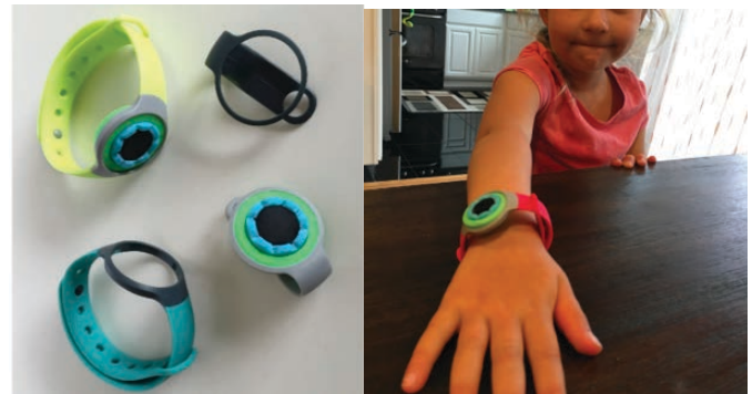
FIG. 4: FINAL WEARABLE DEVICE MODULE PROTOTYPE WITH CIRCULAR SCREEN, ROTATION DIAL, AND PUSH BUTTON
