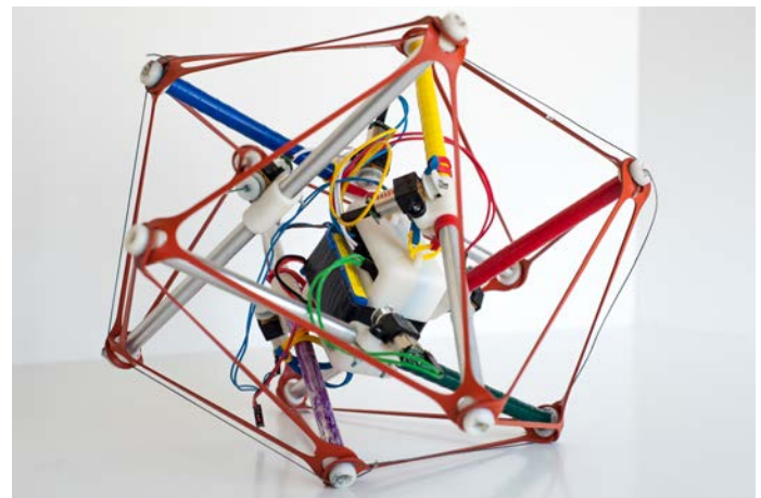
FIGURE 1: The TT-4 mini prototype, the first tensegrity robot that uses the elastic lattice platform. This robot moves by adjusting the lengths of its cables with respect to its elastic lattice.
