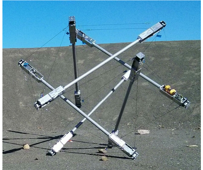
Fig. 1: SUPERball, fully assembled, in the NASA Ames Research Center Roverscape.
