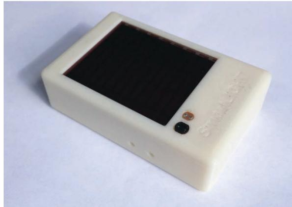
Figure 2: Remote light sensor with Sanyo AM-1815 photovoltaic cell
