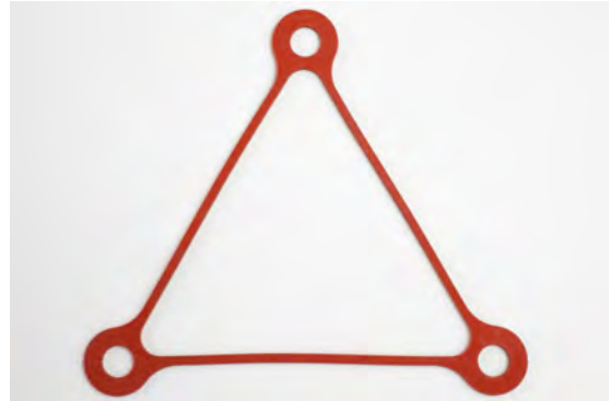
FIGURE 3: Modular elastic lattice prototype made with 60A durometer rubber.
