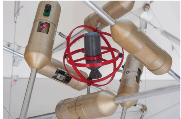
Figure 9. A mockup of a gimbal-enclosed thruster system located at the center of the robot. Red and grey parts are mockups of a gimbal and cold gas thruster, respectively. The gimbal-enclosed thruster is connected to the robot structure with springs.
