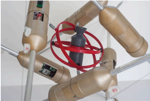
Figure 9. A mockup of a gimbal-enclosed thruster system located at the center of the robot. Red and grey parts are mockups of a gimbal and cold gas thruster, respectively. The gimbal-enclosed thruster is connected to the robot structure with springs.
