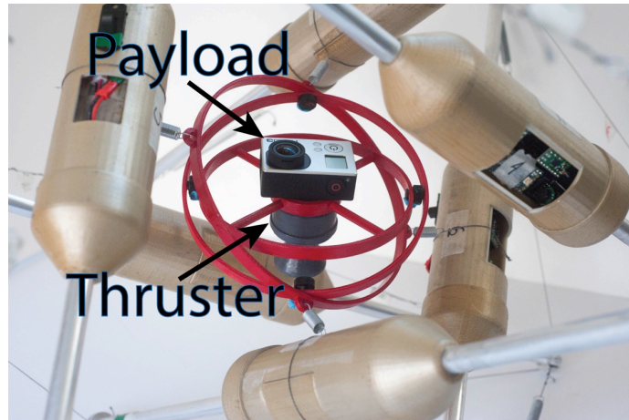
Figure 11. An imaging system was attached to the mockup of a gimbal-enclosed thruster system at the center of the robot to represent the potential payload size and location. With this setup, the imaging equipment or payload can rotate and sweep within the gimbal system.
