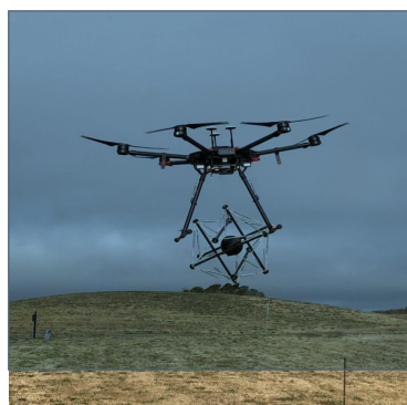
Figure 42. Left: Squishy Robotics’ passive system prototype dropped from a drone. Right: 3D CAD Model of the active system
