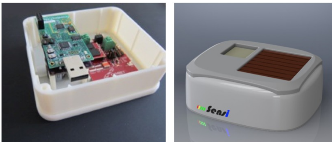
Figure 2. Sensor platform with optional solar panel for energy harvesting
