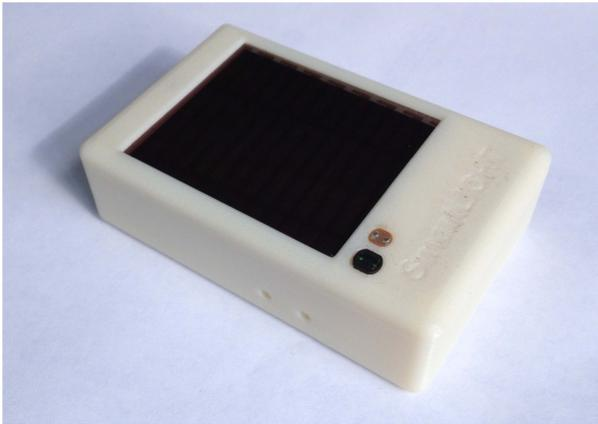
Fig. 2. Remote light sensor with Sanyo AM-1815 photovoltaic cell.
