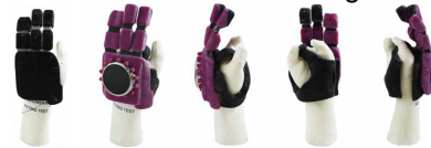
Fig 2. Multi-material printing with standard 3D printer (Ultimaker 3) and industrial grade 3D printer (Objet connex 260)
